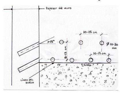
In every drillhole it's necessary to place an injection rod and the product will be injected with 5-6 bar pressure.
